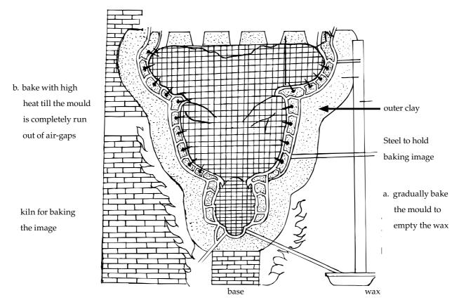
Fig. 6: Emptying beeswax from the mould
